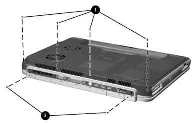
Removing the Keyboard Cover Screws
